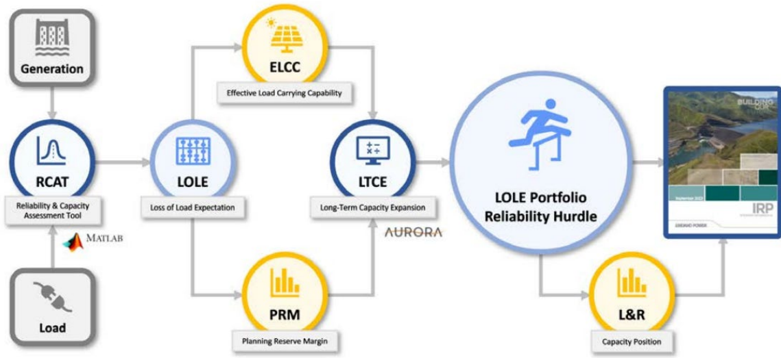
1 Figure 1. Idaho Power's Reliability Flowchart
